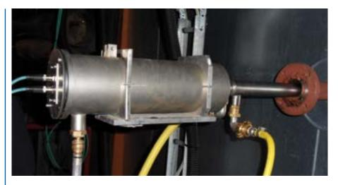
The answer to this measurement and analyzing task is the D-VTA 200-Mobile system. The D-VTA 200-Mobile system is the adaptable, not fixed stationary installed Combustion analysis system based on optical analysis of the combustion process.
