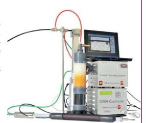
The sampling probe (Ø 8 mm) is designed for direct connection to stacks. Since both dilution stages employ 9 lpm dilution air, the dilution ratio depends on the volume flow rate of the measuring system. For example, at a sample flow of 1 lpm it equals 1:10 or, if the second dilution stage is used, 1:100. Other dilution ratios are available upon request.
